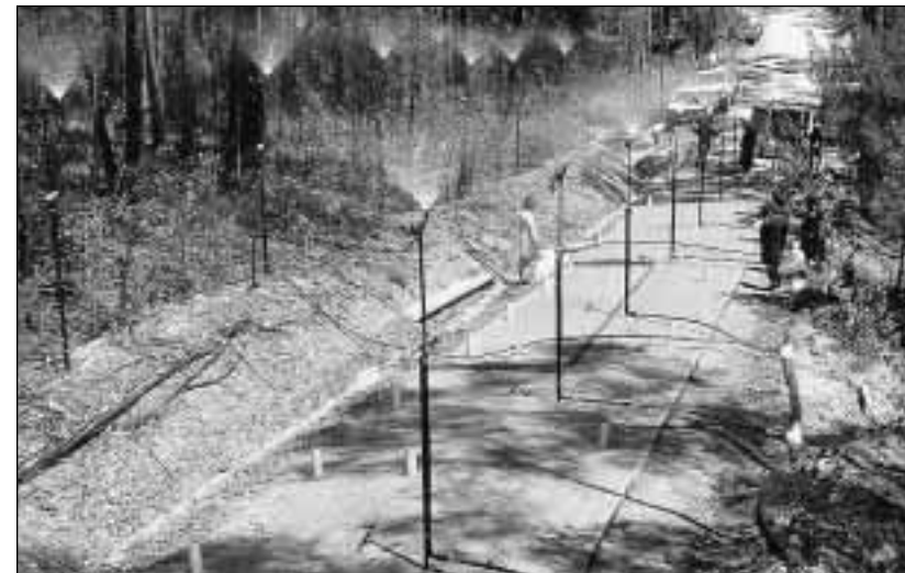
Rainfall simulation along ridgetop road in Cuttagee Creek covering an area of 300-600 m 2 , with a contributing road length of 40 m
