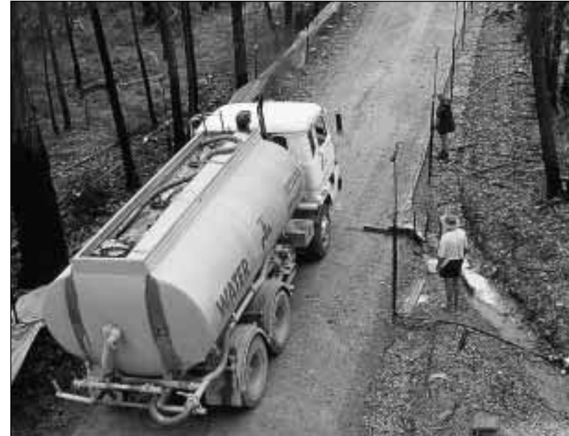
The dramatic effect of traffic intensity on sediment production from forest roads - a heavy water-truck pounds the surface of an experimental site in Cuttagee Creek, near Bermagui
