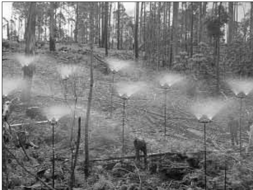
Rainfall simulation on logged snig track and general harvesting area, Eden Forest Management Area, NSW
