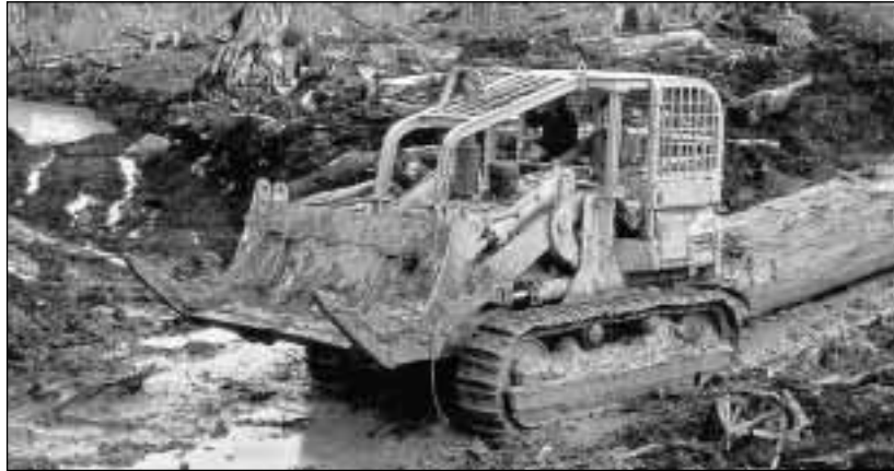
Heavy logging machinery causes soil and vegetation disturbance, especially during wet weather
