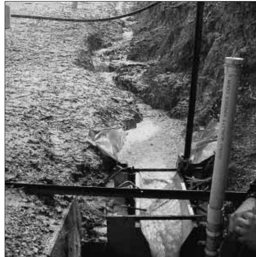
Runoff being measured in a flume on a road segment in Cuttagee Creek - note water concentration in roadside ditch
